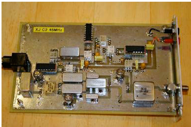
Figure 5: picture of the 45 MHz synthesis board
