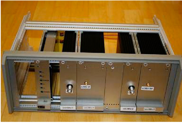
Figure 9: picture of the realized pre-multiplier
